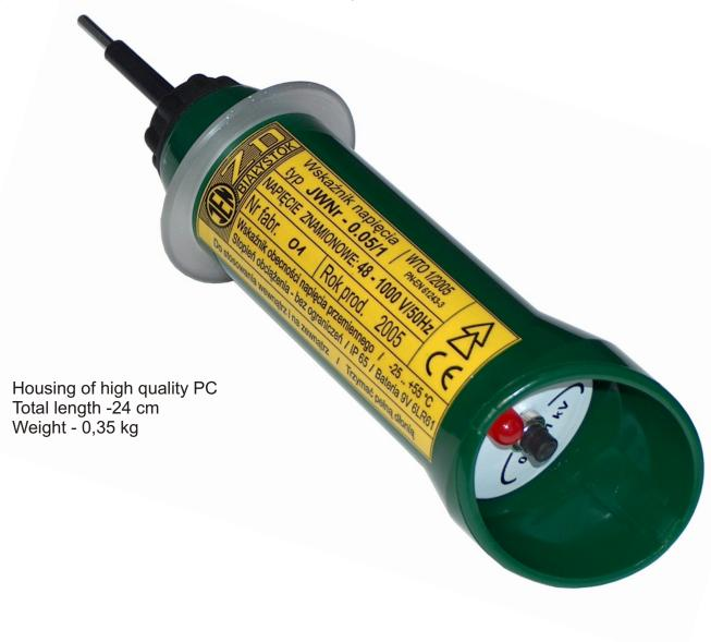
Operating and efficient indicator produces periodical audio and light signals. Voltage control is carried out in the way of touching to examined area with the contact stud. In case the place is under voltage, periodical audio and light signals change into constant.
